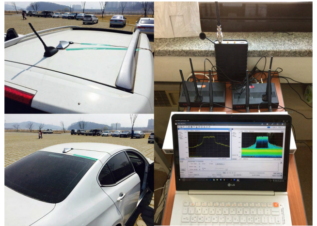
FIGURE 1. Measurement campaign for channel measurements in vehicular environments. Each vehicle is equipped with off-the-shelf OBU and the antenna mounted on the roof of the car. A signal power-triggered spectrum analyzer is installed at the receiving end.
