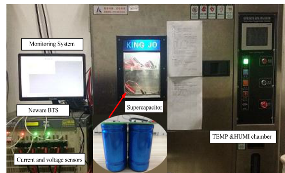
FIGURE 8. Multi-channel test platform of the SC.
