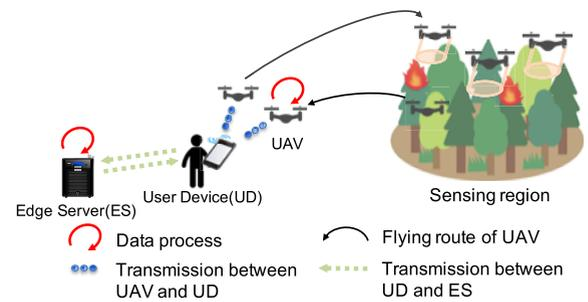
FIGURE 1. Diagram of multi-UAV search system.
