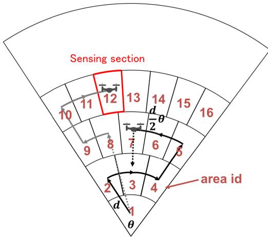
FIGURE 4. Sensing region of two-dimensional model.
