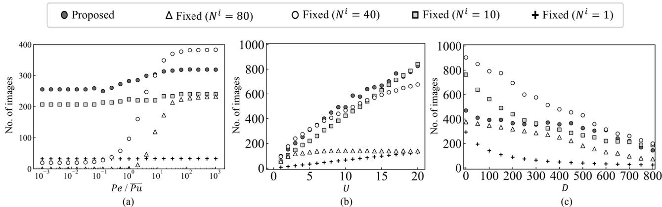
**FIGURE 6.** No. of images that had shorter ETA than 120 s at 600 s after start time. (a) Processing speed of ES vs. no. of images. (b) No. of UAVs vs. no. of images. (c) Distance between initial position and center of sensing block where area id is 1 vs. no. of images.
