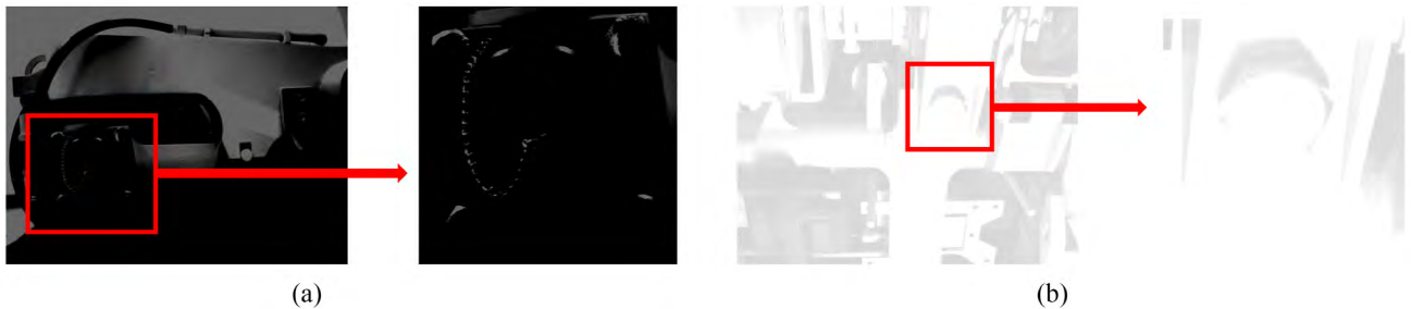
FIGURE 15. Images with undetected key component regions. (a) The image under extremely low lighting condition. (b) The image under bright illumination.
