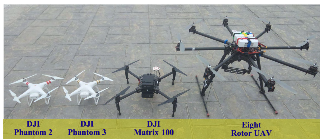
FIGURE 14. Experimental UAVs with different appearances and sizes, including DJI Phantom 2, DJI Phantom 3, DJI Matrix 100 and eight-rotor UAV.
