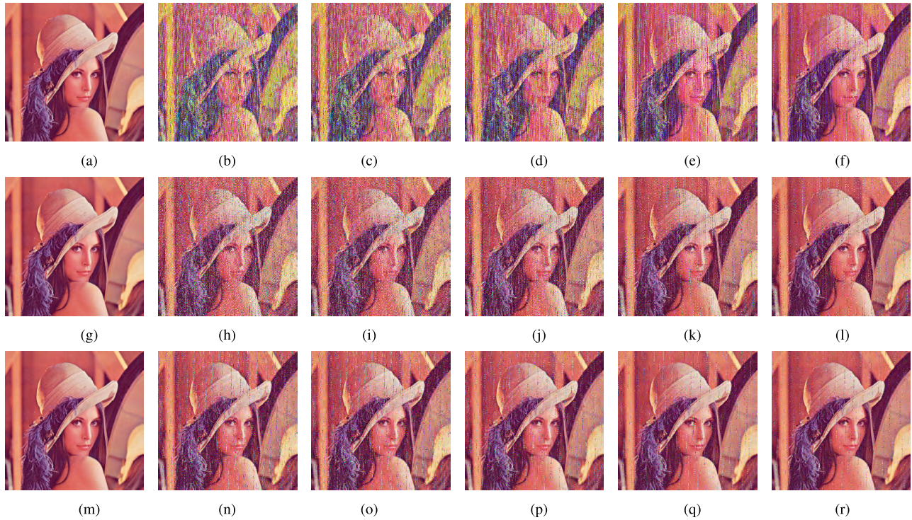
FIGURE 23. An example of image transmission with Lena (the pixel size is 256 \times 256 ) is applied to visualize the impact of different modulation schemes for various methods in the UWA-OFDM system over channel-II, where the value of SNR is also set to 20 dB. The first column shows the original transmitted images. The second to sixth columns show the reconstructed results from LS, BPNN, the proposed DNN-1, DNN-2, and MMSE methods. The original image data are modulated with 64QAM, 32QAM, and 16QAM in these three rows, respectively. (a) original. (b) LS(64QAM). (c) BPNN(64QAM). (d) DNN-1(64QAM). (e) DNN-2(64QAM). (f) MMSE(64QAM). (g) original. (h) LS(32QAM). (i) BPNN(32QAM). (j) DNN-1(32QAM). (k) DNN-2(32QAM). (l) MMSE(32QAM). (m) original. (n) LS(16QAM). (o) BPNN(16QAM). (p) DNN-1(16QAM). (q) DNN-2(16QAM). (r) MMSE(16QAM).
