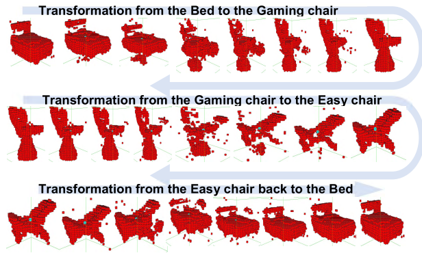
FIGURE 16. Centroid-based interpolation: First, the centroids of the three clusters to be interpolated are selected. Then, the nearest sample code from an individual centroid is selected, as exemplified in the figure with a bed, gaming chair, and easy chair. The transformation from the bed to the gaming chair is shown in the first row, where the first sample shows the starting point of interpolation and the last sample shows the interpolated sample by changing its feature code in the response field. The in-between samples show the intermediate representation of the transformation from the bed to the gaming chair. The first sample of the second row shows the last interpolated sample from the bed, which is the gaming chair, and this is transformed to the easy chair, whereas the first sample of the last row is the result of interpolation from the gaming chair to the easy chair, where it is transformed back to the bed.
