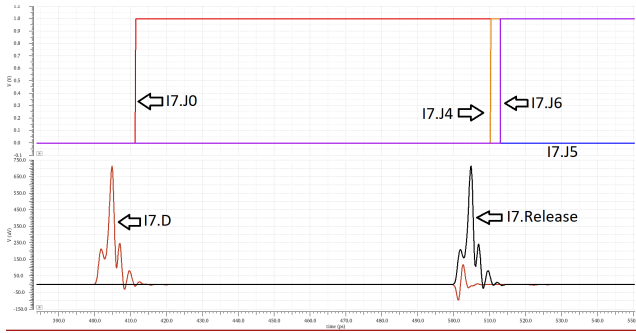
FIGURE 17. Correct action of the DFFR 17. 17.J5 does not increment.
