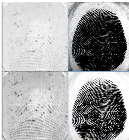
FIGURE 5. Image contrast enhancement by Gamma correction. Top row: input image; bottom row: enhanced images, column-wise, respectively.
