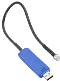
FIGURE 4. 3-array MOS gas sensor array signal acquisition board.
