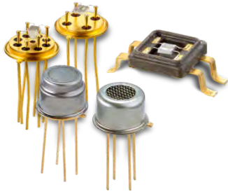
FIGURE 3. 3-array MOS gas sensor.
