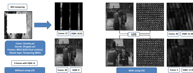
FIGURE 6. Recovering the secret video “Chappie.avi” with and without using LCG randomization technique after tampering the “Gravity.avi” stego video with a white box that covers 80% of each of the stego video frames.
