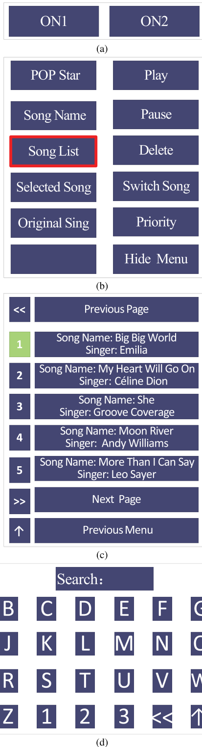
FIGURE 6. The four types of sub-GUIs in the music-on-demand system: (a) system switch (sub-GUI0). (b) main menu (sub-GUI1). (c) song list menu (sub-GUI4, sub-GUI5 and sub-GUI6). (d) song search menu (sub-GUI2 and sub-GUI3).
