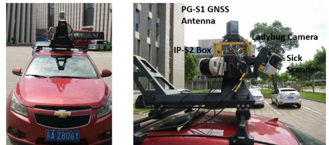
FIGURE 2. Components of the 3D mobile mapping system.
