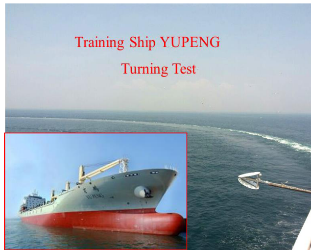
FIGURE 2. Turning test of the training ship YUPENG.
