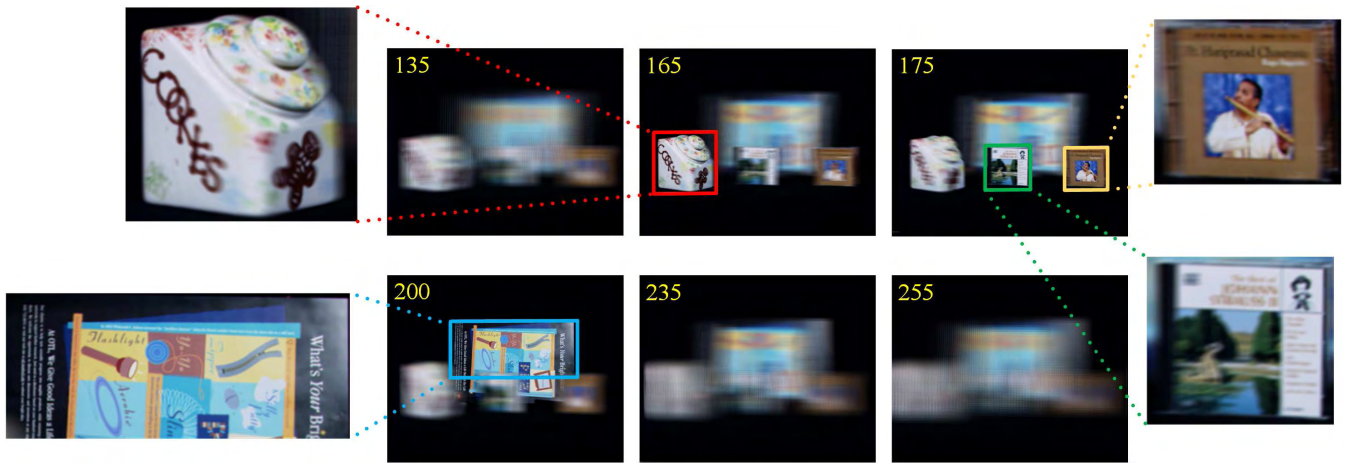
FIGURE 7. Samples of synthetic aperture images utilized in the Stanford CD-case scene. The relative focusing depth increases from top left to bottom right. The result of this scene is shown in Table 3.
