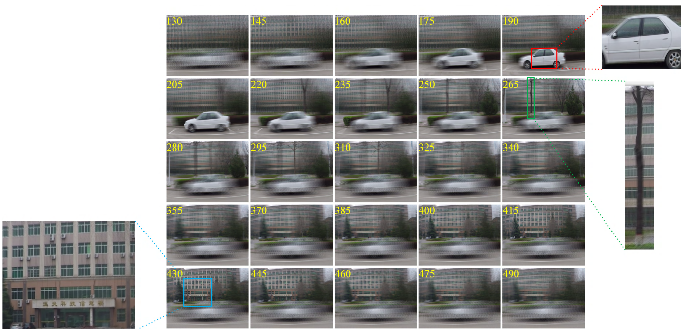
FIGURE 8. Synthetic aperture imaging results of focusing at increasing relative depths from top left to bottom right. The top left image is focused at 130 relative depth and the bottom right image is focused at 490 relative depth. Images focused at 190 depth (row 1, column 5) and 430 depth (row 5, column 1) appear sharp while others appear blurry. The curve of auto-focusing in this scene is shown in Fig. 9.
