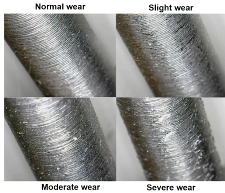
FIGURE 6. Four tool wear levels based on the degree of roughness on workpiece surface.
