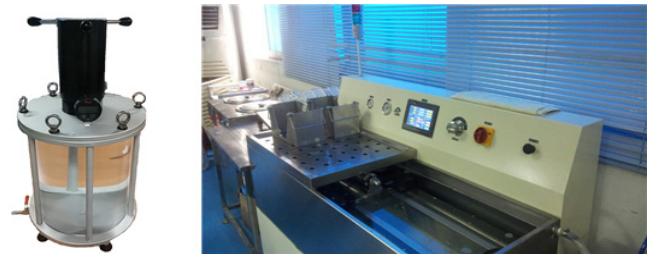
FIGURE 12. Waterproof test instrument used for functional evaluation.
