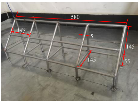
FIGURE 10. Reduced-scale PV framework model, unit(mm).
