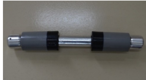
FIGURE 3. Figure of the cable installed with a stress cone.
