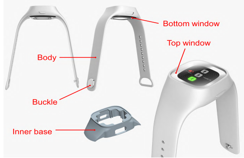
FIGURE 4. Our designed appearance schematics of the wearable device.
