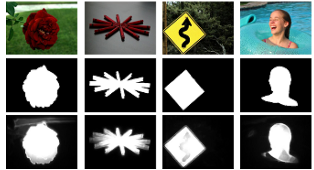
FIGURE 2. Saliency detection results: the first row is original images, the second row is ground truth and the third row is saliency map.
