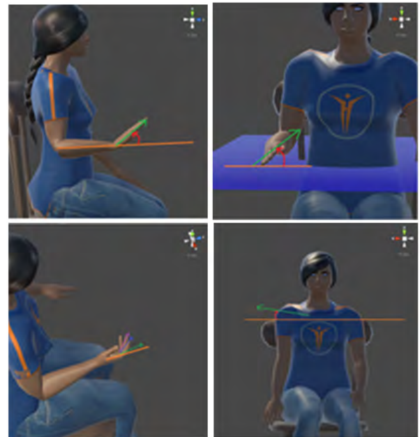
FIGURE 5. The angles considered for evaluating the Palm flexion-extension (top-left), Forearm pronation-supination (top-right), Finger flexion-extension (bottom-left) and Shoulder raise movements (bottom-right).
