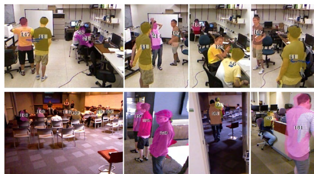
FIGURE 16. People detection and tracking results on office dataset (first row) and mobile camera dataset (second row) [166].
