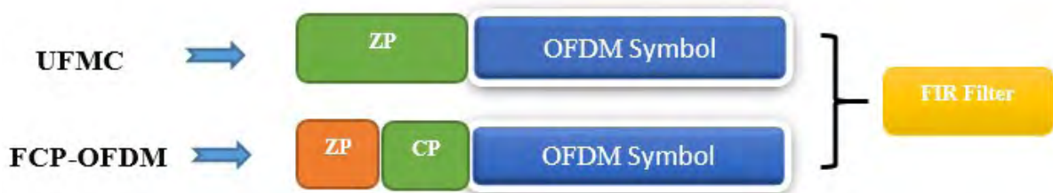
FIGURE 9. The difference between FCP-OFDM and UFMC.
