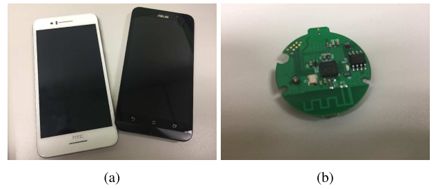
FIGURE 6. Experimental devices. (a) The training and the operating mobile devices: HTC Desire 728 and ASUS ZE551ML. (b) The beacon device.
