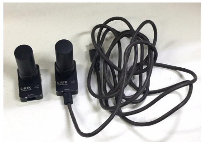
FIGURE 10. RTK system is used to obtain the precise altitude of the quadrotor UAV.
