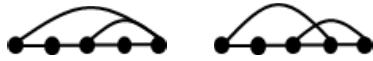
FIGURE 2. Example of an outerplanar motif where edges do not intersect (left) and the non-outerplanar alternative (right). HVG motifs are outerplanar.
