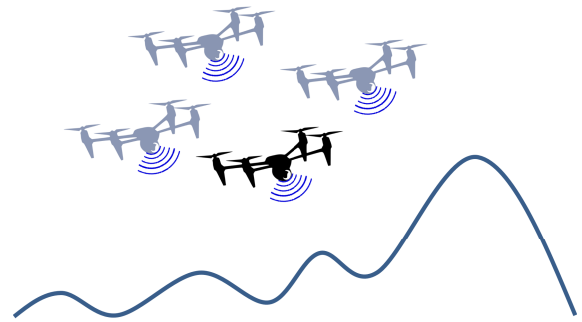
FIGURE 1. Leader-follower formation tracking of four under-actuated VTOL UAVs. They are cooperatively conducting a surface inspection task. The dark UAV serves as the leader and the others are the followers.
