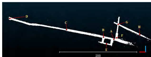
FIGURE 13. The top-view of the map generated by NDT-SLAM with several scan poses. The robot started at point A and followed this sequence A-B-C-B-D-C-B-E-A-F-G-H. Stationary reflective markers were arranged at cross of A, C, D, F, G.
