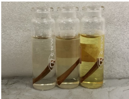
FIGURE 9. The insulation oils with different aging time.
