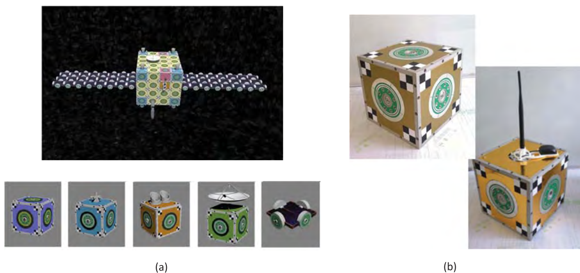
FIGURE 2. (a) Cellular satellite developed by NWPU. (b) Prototypes of two unit cells.
