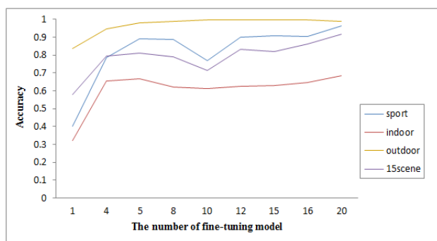
FIGURE 5. The trend of classification accuracy is obtained by our model which is fine-tuned in different interval on four scene datasets.
