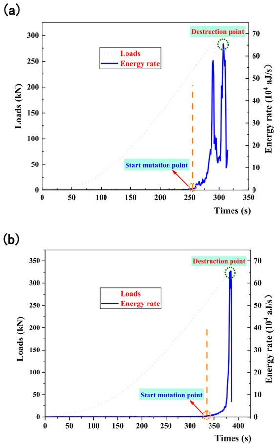
**FIGURE 1.** Characteristics of acoustic emission energy rate changes of different specimens (a) Specimen 1 (b) Specimen 2.
