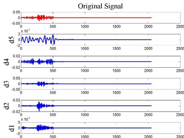
FIGURE 8. Waveform signals decomposed at different scales.
