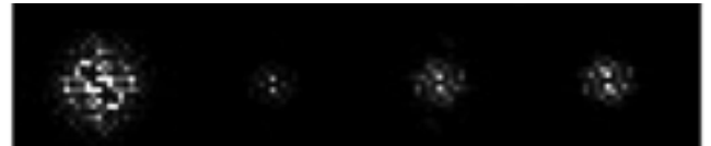
FIGURE 15. Measured NPS of the CT images of the laboratory mouse in Fig. 12: (a) the high-resolution image as the reference, (b) the low-resolution image to be processed, (c) the deblurred slice using the proposed method, (d) the deblurred image using the 3D image domain method. Zero frequency is at the center of each NPS.
