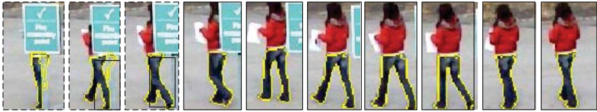
FIGURE 3. These figures are 10 detections in continuous frames, where solid rectangular boxes are the detections produced by the detector and dashed rectangular boxes are the rediscovered detections produced by our approach. The regions surrounded by yellow curves form a supervoxel.
