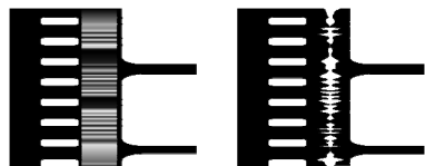
FIGURE 50. Variable-area (left) and variable-density (right) sound-on-film (SOF) systems.
