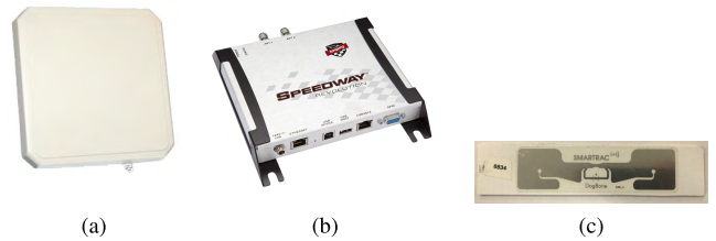
FIGURE 3. RFID System installed on Doris. (a) Antenna. (b) Impinj R220 Reader. (c) RFID tag dogbone.
