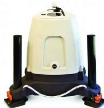
FIGURE 1. ZephIR 300 Onshore Wind Lidar.
