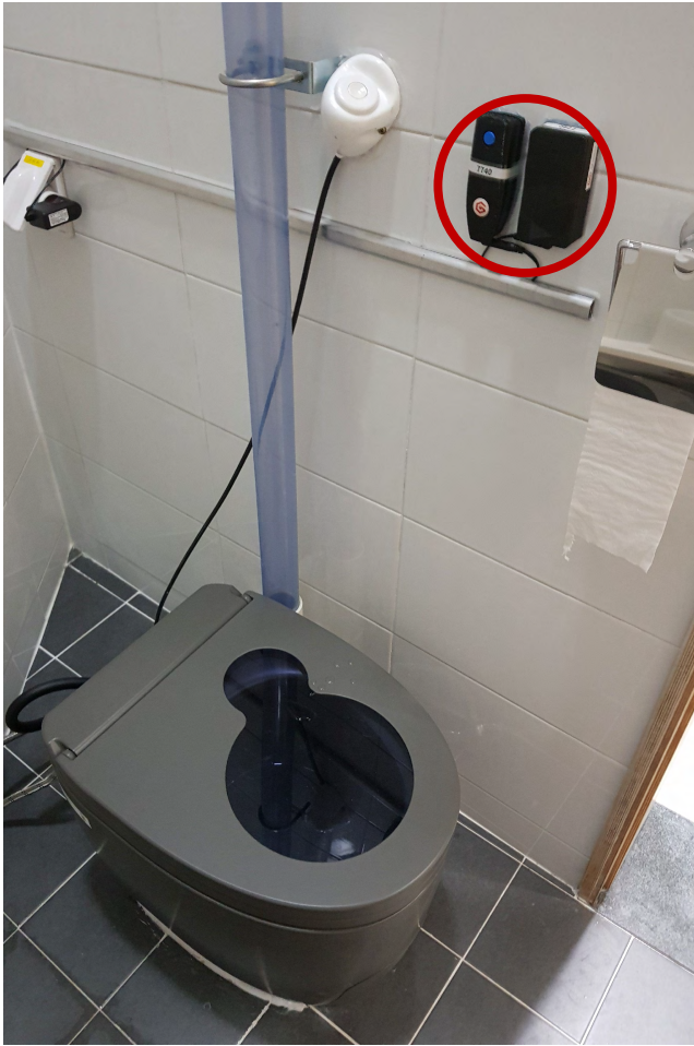
FIGURE 17. The smart toilet and BLE communication device.
