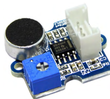
FIGURE 4. The added sound sensor to increase the accuracy of measurement.
