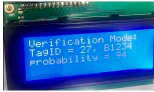
FIGURE 10. An example of tag detected with positive predictive value of 94, taken from confusion matrix.
