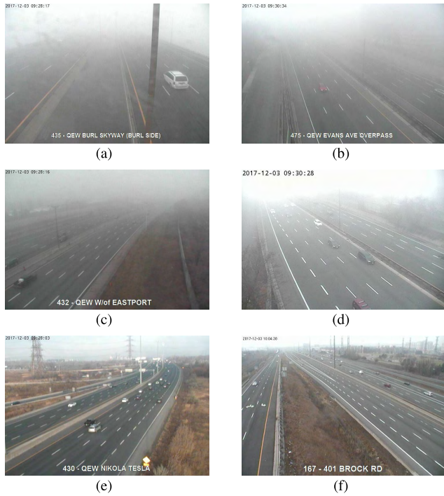
FIGURE 7. Sample of the captured foggy images for the practical visibility distance measurements, their measured visibility distances are 38 m, 64 m, 73 m, 168 m, 296 m and 358 m, respectively.
