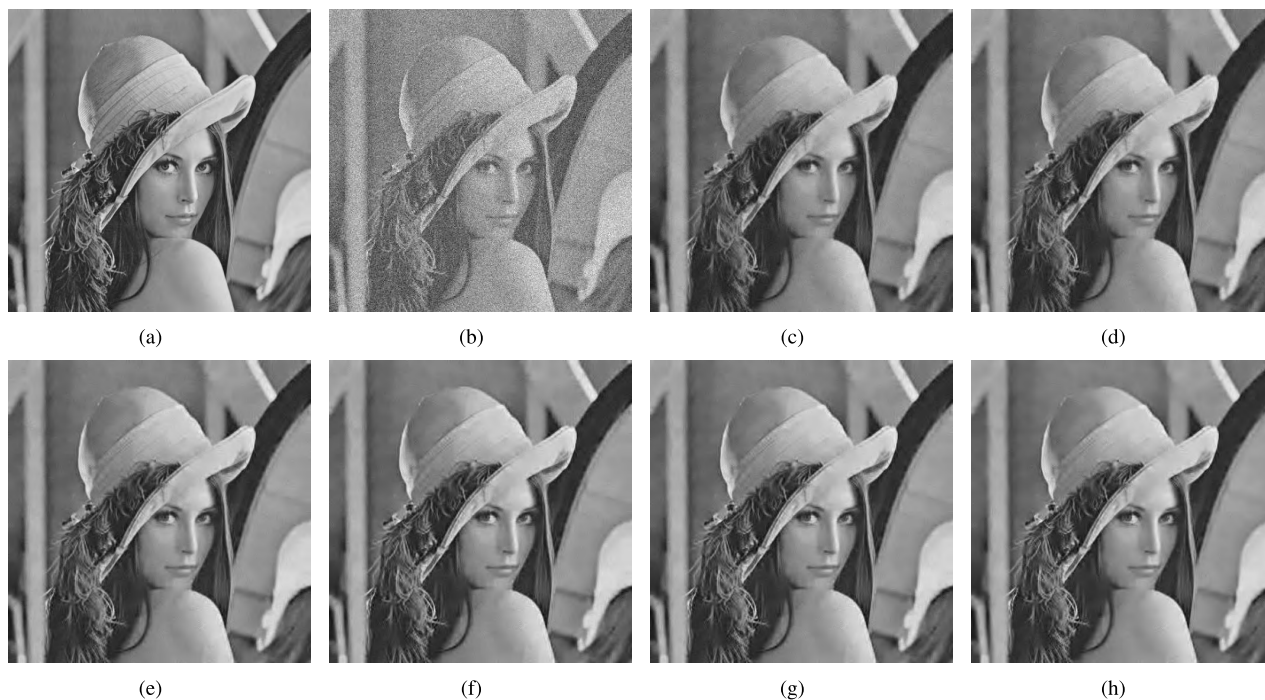
FIGURE 9. Image-denoising result: (a) Original image; (b) Noised: 20.17 dB; (c) ISTA: 29.13 dB; (d) WISTA0.9: 29.88 dB; (e) WISTA0.7: 30.79 dB; (f) WISTA0.5: 31.01 dB; (g) IHITA: 31.00 dB; and (h) OMP: 30.93 dB (from top left to bottom right)
