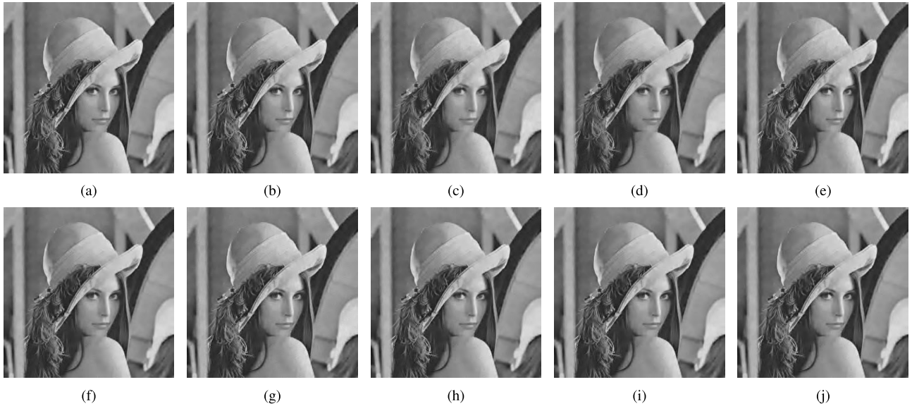
FIGURE 10. Image-denoising result with DNN-SC algorithms: (a) LISTA: 29.71 dB; (b) TISTA: 29.37 dB; (c) LWISTA0.9: 29.89 dB; (d) TWISTA0.9: 29.69 dB; (e) LWISTA0.7: 30.45 dB; (f) TWISTA0.7: 30.47 dB; (g) LWISTA0.5: 30.68 dB; (h) TWISTA0.5: 30.76 dB; (i) LIHTA: 30.82 dB; and (j) TIHTA: 30.80 dB (from top left to bottom right).
