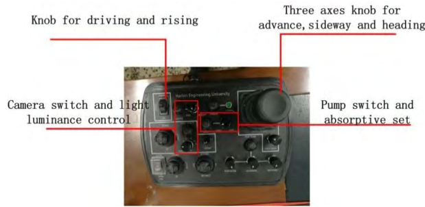
FIGURE 4. Function assignment of the joystick.
