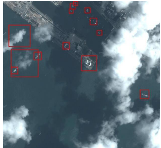
FIGURE 5. Result of ship candidate extraction, including real ships and background regions.
