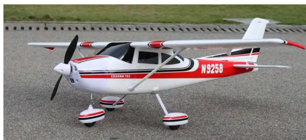
FIGURE 1. Scale Cessna 182 – 1/6.65 ratio to the Prototype Cessna 182 [9].
