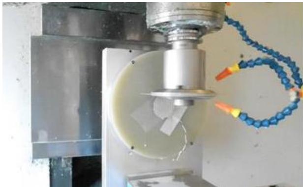
FIGURE 6. Picture of the dicing process of the ceramic. The ceramic is attached to a sacrificial plate and diced using a diamond blade in the CNC.
