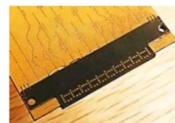
FIGURE 15. Geometry of magnetoelectric dipole loaded SIW horn antenna and array [33].
