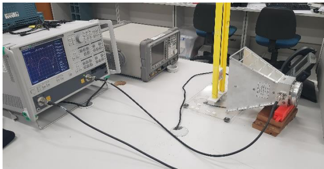
FIGURE 19. The tag measurement setup.
