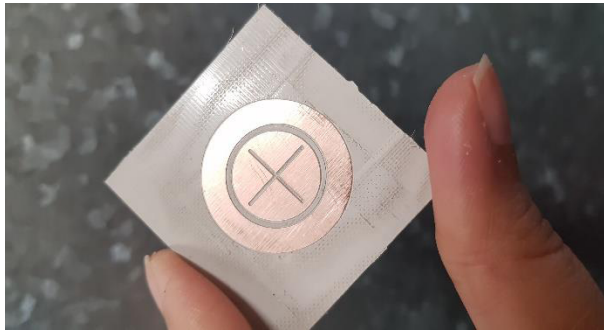
FIGURE 18. The fabricated tag on Taconic Cer-10 that is corresponding to the tag ID 010001100. D2 = 9.18 mm, W2 = 0 mm, L1 = 12.4 mm, L2 = 11 mm, and W1 = 0.4 mm.
