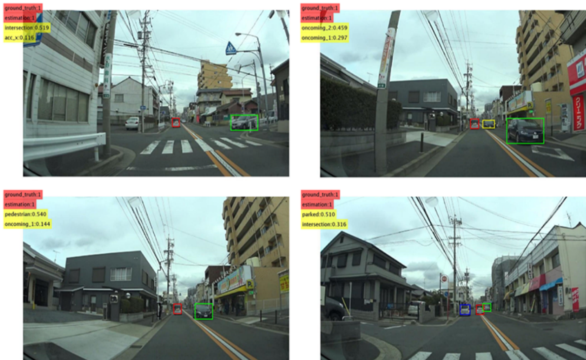
FIGURE 20. Samples of true risk perception correlated to images of traffic conditions(Upper left: risk predicted in intersection; Upper right: risk from the second opposite vehicle; Bottom left: risk from the roadside pedestrian; Bottom right: risk from the front parked vehicle).
