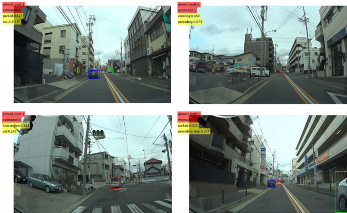
FIGURE 21. Samples of true risk perception correlated to images of traffic conditions(Upper left; risk from the parked vehicle. Upper right; risk from the merging vehicle. Bottom left; risk from the crossing intersection. Bottom right; risk from the parked vehicle).
