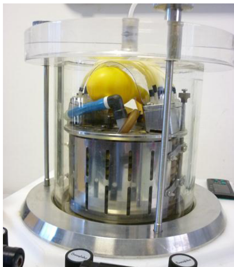
FIGURE 3. The physical model: the yellow balloon is used to model the interstitial volume and is connected to the capillary bed through valve V5 of Fig. 1.
